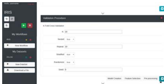
Figure 2: UI - Showing cross validation task (a validation procedure task) and the tasks that can be used after.
